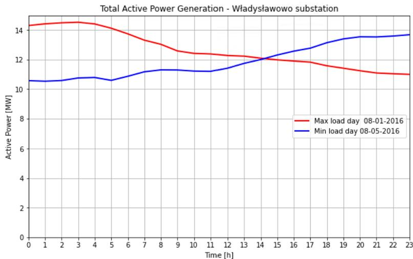
*Figure 2.3 Total Active Power Generation Max and Min load days*
