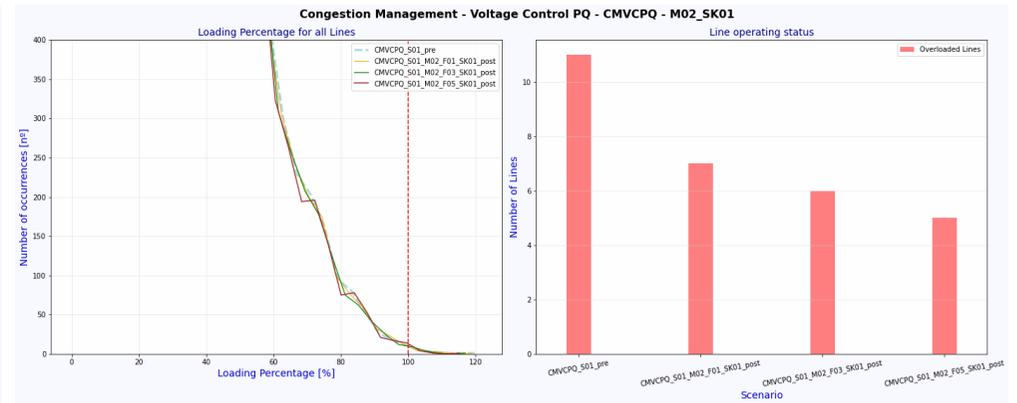
**Figure 2.35 Deviation plots for Loading Percentage [%] of all lines obtained from Congestion Management - Voltage Control with Active and Reactive Power (a) Scenario M01-K01, (b) Scenario M02-K01. Scenario 1, DE-NET1-LV.**
