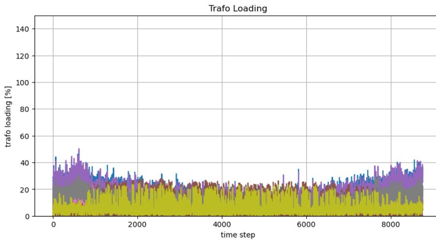
*Figure 2.25 Transformers loading [%] for the Scenario 0, DE-NET1-LV*
