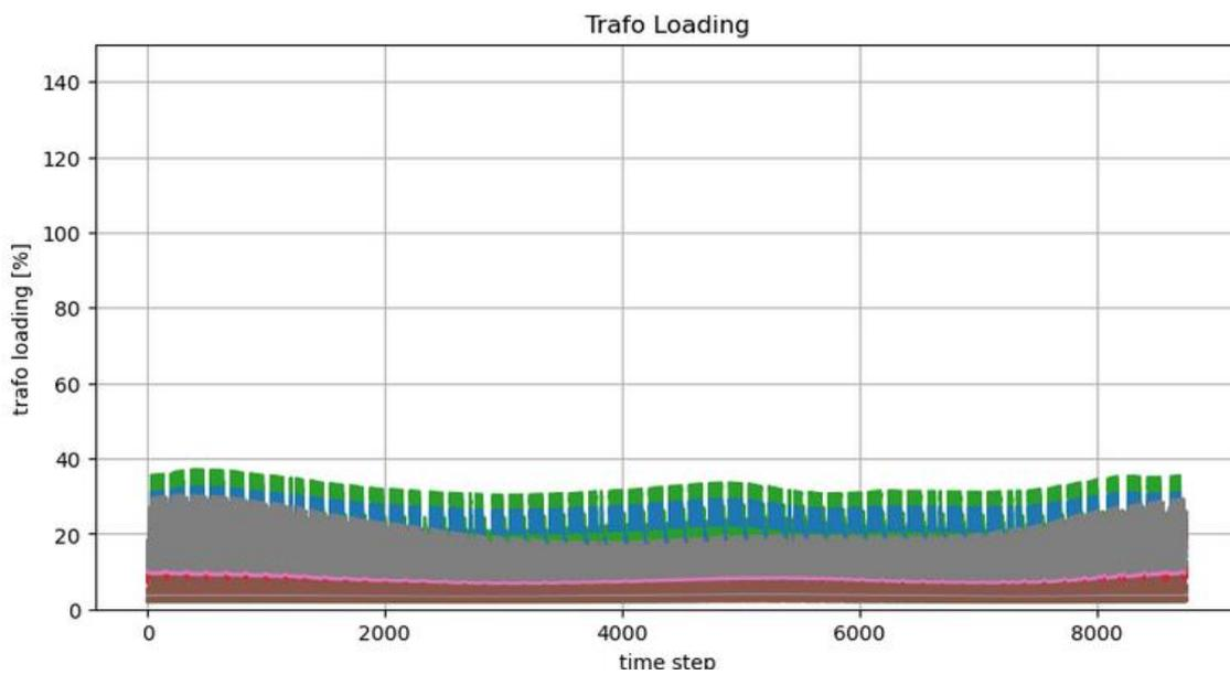
*Figure 2.57 Transformer loading [%] for the Scenario 1, PT-NET1-MV-LV*
