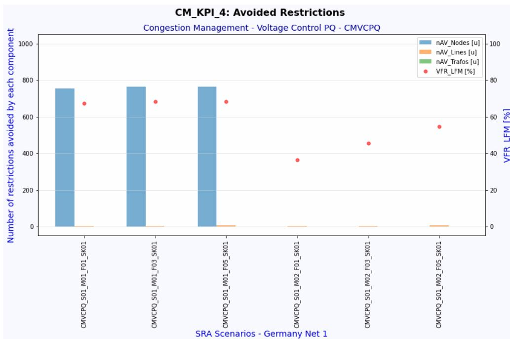
Figure 2.38 KPI CM\_SPI\_4: Avoided Restrictions for Congestion Management, Voltage Control using Active or Reactive Power (CMVCPQ)
