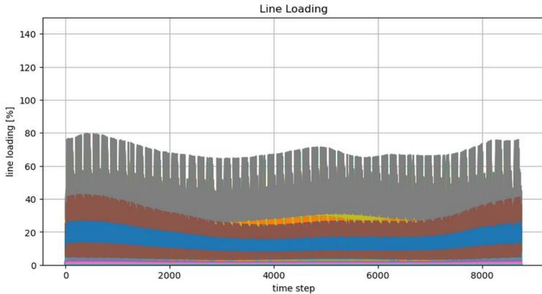
*Figure 2.53 Lines loading [%] for the Scenario 0, PT-NET1-MV-LV*
