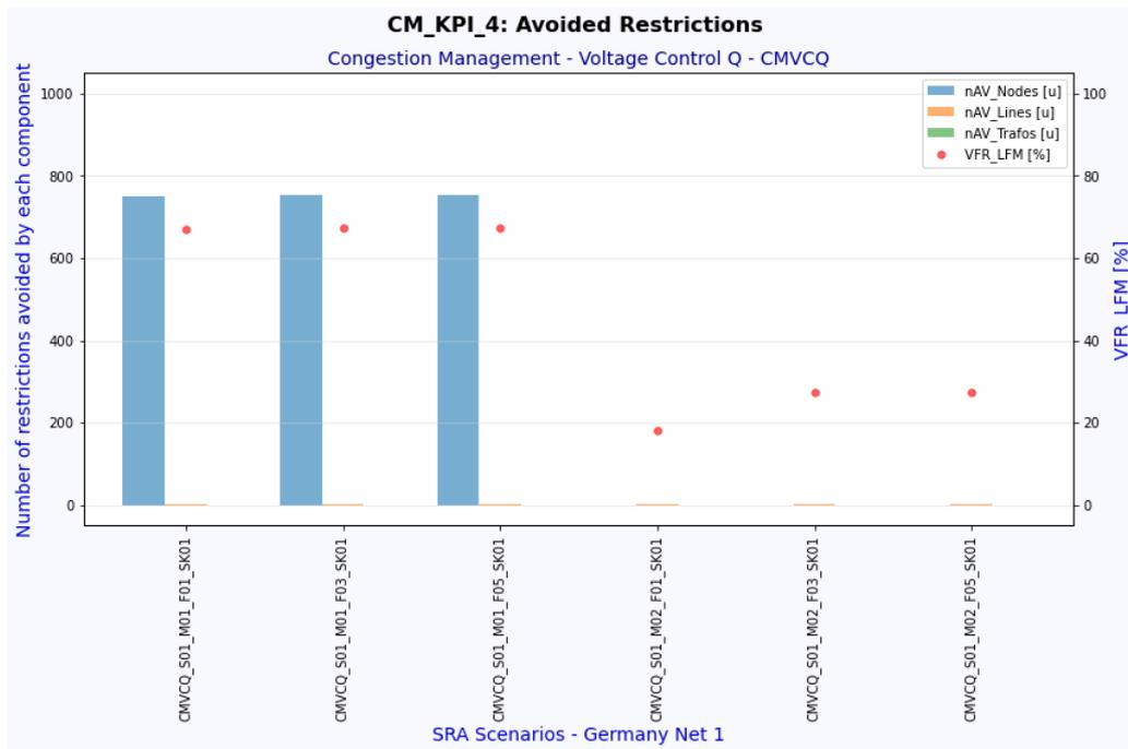
Figure 2.37 KPI CM\_SPI\_4: Avoided Restrictions, for Congestion Management, Voltage Control using Reactive Power (CMVCQ)
