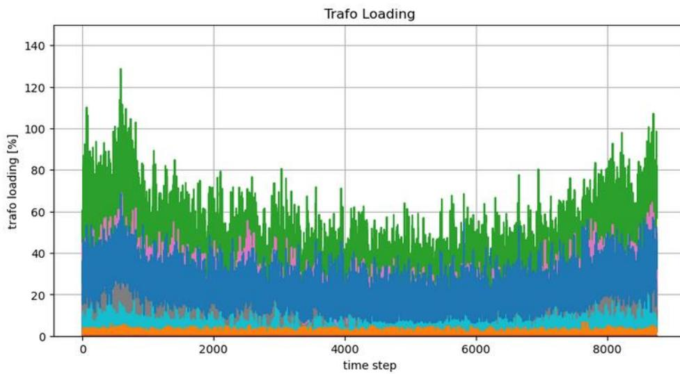
*Figure 2.41 Transformer loading [%] for the Scenario 0, DE-NET2-LV*
