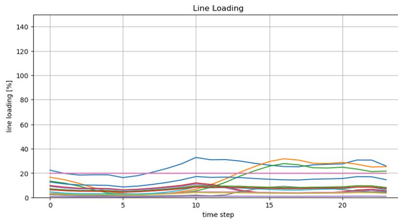
*Figure 2.7 Line loading [%] for the Scenario 0, min load day, PL-NET1-MV*
