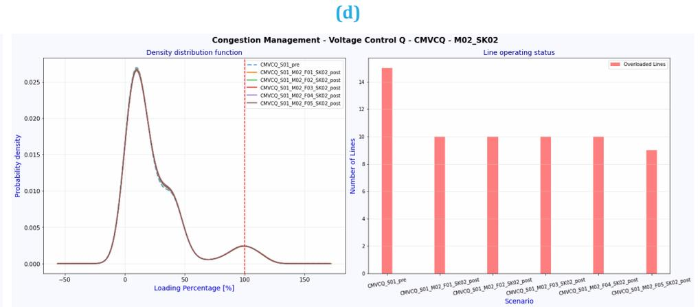
**Figure 2.18 Density plots for Loading Percentage [%] of all lines obtained from Congestion Management – Voltage Control with Reactive Power (a) Scenario M01-K01, (b) Scenario M02-K01, (c) Scenario M01-K02, (d) Scenario M02-K02. Scenario 1, PL-NET1-MV**
