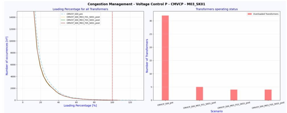
Figure 2.46 Deviation plots for Loading Percentage [%] of all Transformers obtained from Congestion Management – Voltage Control with Active Power (a) Scenario M02-K01, (b) Scenario M03-K01. Scenario 0, DE-NET2-LV.
