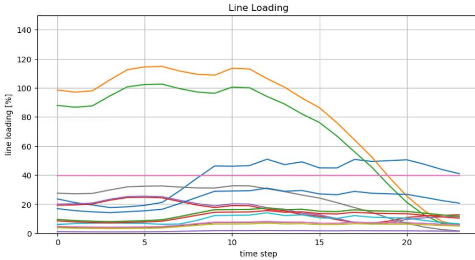
**Figure 2.10** Line loading [%] for the Scenario 1, PL-NET1-MV
