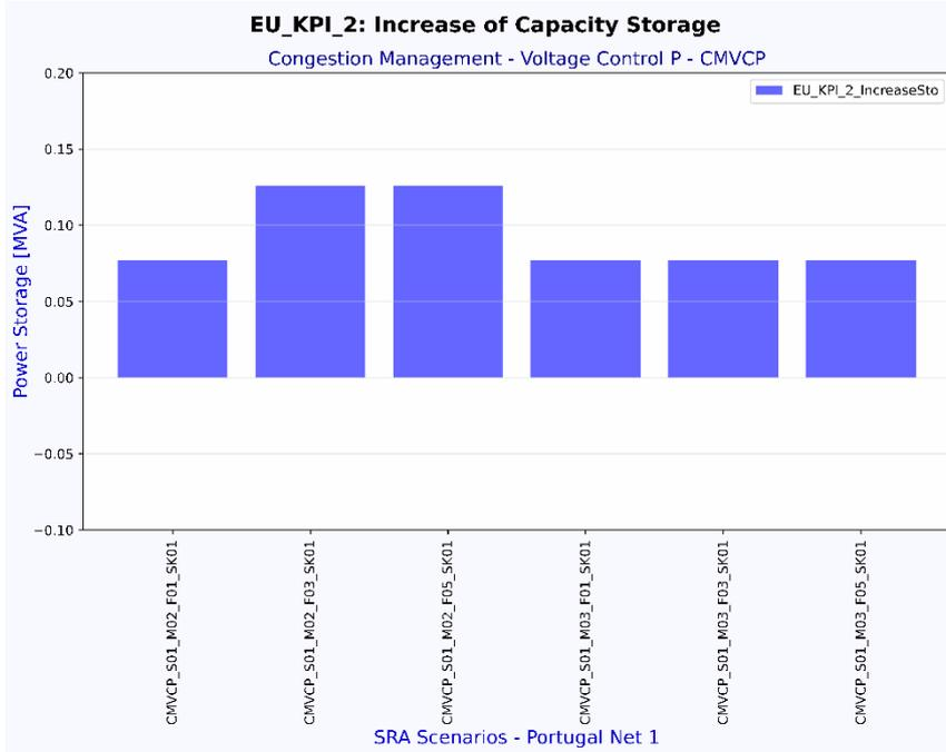
**Figure 2.113 EU\_KPI\_2: Increased of capacity storage solution, for Congestion Management, Voltage Control using Active Power (CMVCP)**
