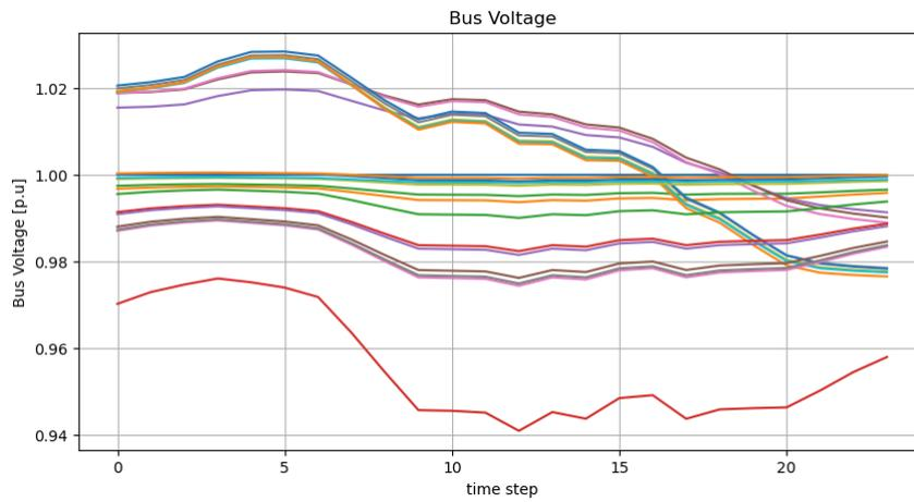
*Figure 2.6 Bus Voltage [p.u.] for the Scenario 0, max load day, PL-NET1-MV*
