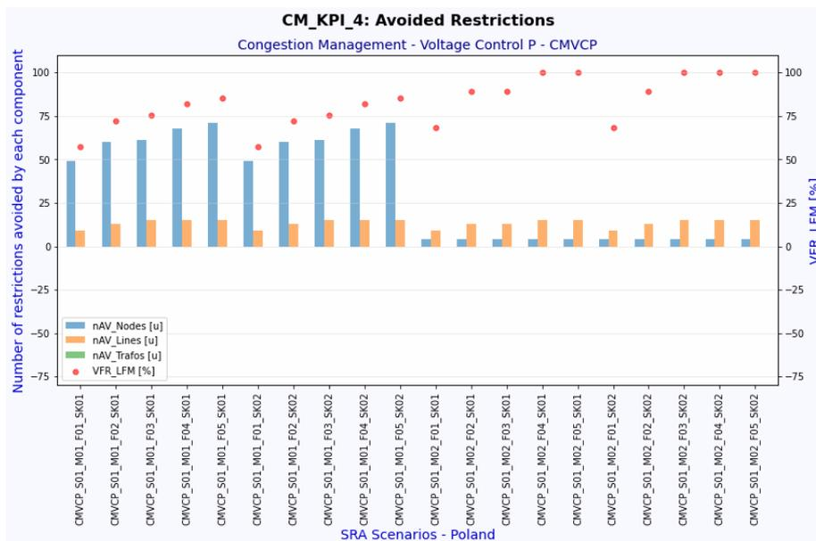
Figure 2.20 KPI CM\_SPI\_4: Avoided Restrictions, for Congestion Management, Voltage Control using Active Power (CMVCP)
