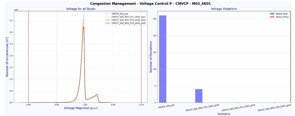
**Figure 2.43** Deviation plots for Voltage Magnitude [p.u.] obtained from Congestion Management – Voltage Control with Active Power (a) Scenario M02, (b) Scenario M03. Scenario 0, DE-NET2-LV.
