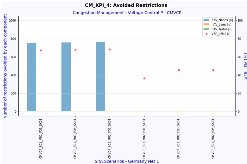
**Figure 2.36 KPI CM\_SPI\_4: Avoided Restrictions for Congestion Management, Voltage Control using Active Power (CMVCP)**
