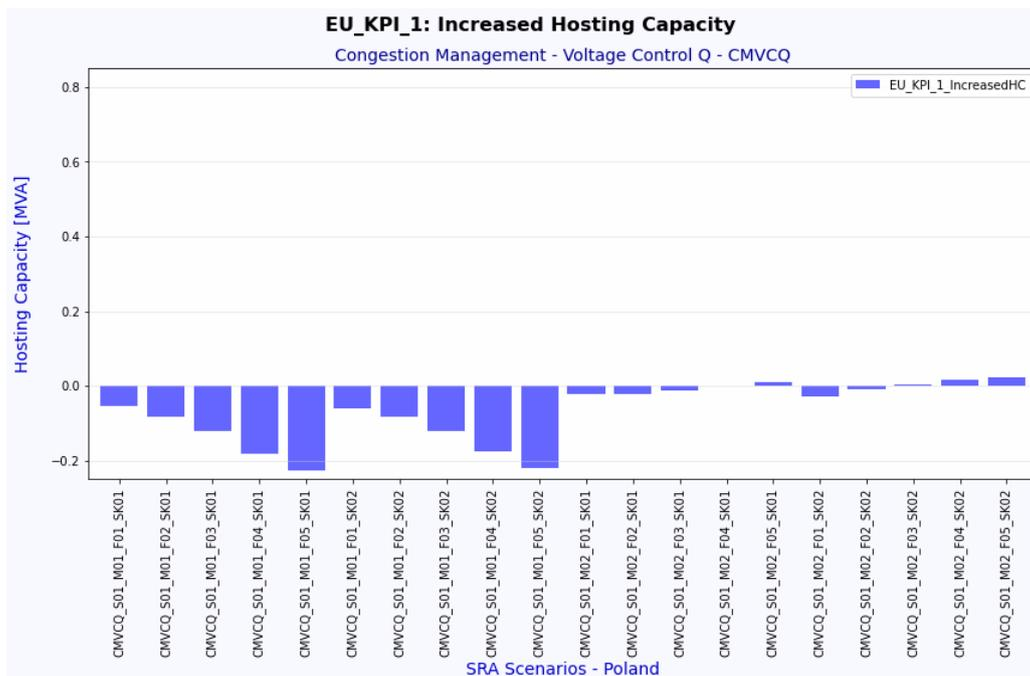
**Figure 2.74 EU\_KPI\_1: Increase Hosting Capacity, for Congestion Management, Voltage Control using Reactive Power (CMVCQ)**
