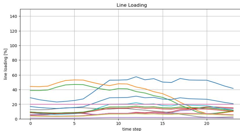
*Figure 2.4 Lines loading [%], Scenario 0, max load day, PL-NET1-MV*
