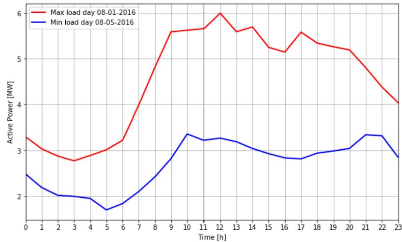
*Figure 2.2 Total Active Power Consumption Max and Min load days*
