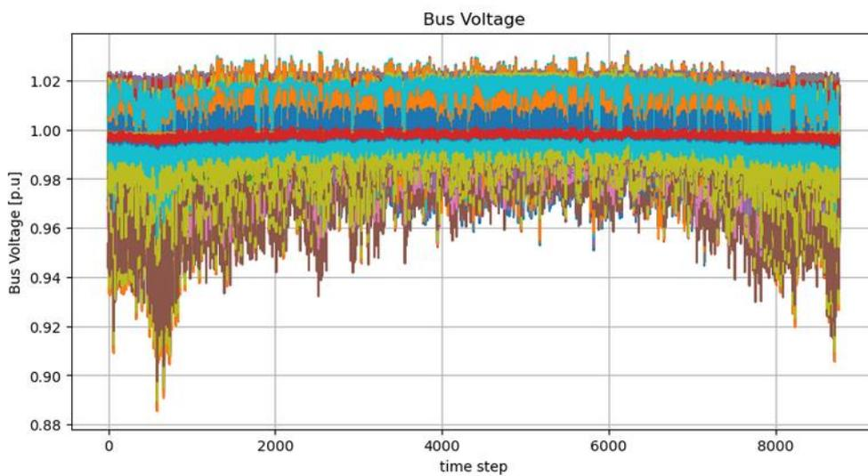
*Figure 2.42 Bus Voltage [p.u.] for the Scenario 0, DE-NET2-LV*
