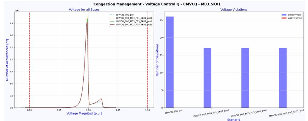
**Figure 2.44** Deviation plots for Voltage Magnitude [p.u.] obtained from Congestion Management – Voltage Control with Reactive Power (a) Scenario M02, (b) Scenario M03. Scenario 0, DE-NET2-LV.
