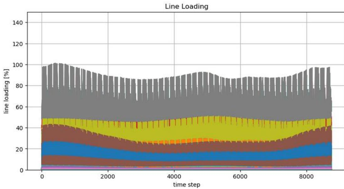
*Figure 2.56 Lines loading [%] for the Scenario 1, PT-NET1-MV-LV*
