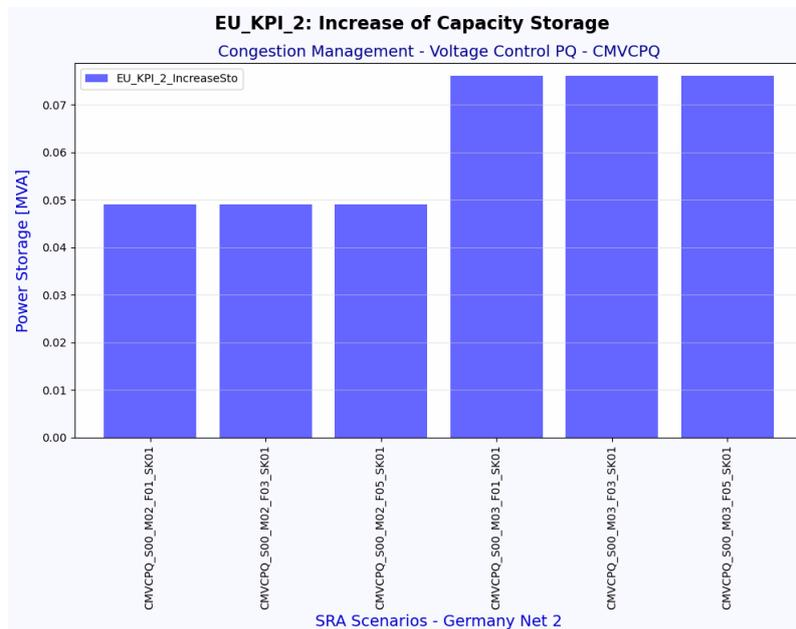
**Figure 2.107 EU\_KPI\_2: Increased of capacity storage solution, for Congestion Management, Voltage Control using Active and Reactive Power (CMVCPQ)**
