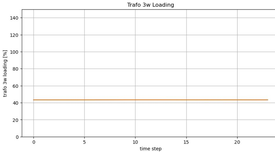
**Figure 2.11** Transformer loading [%] for the Scenario 1, PL-NET1-MV
