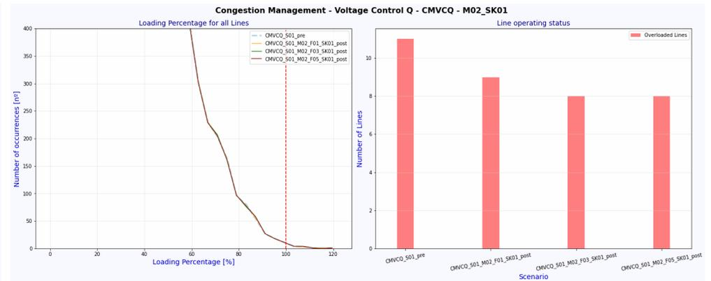
**Figure 2.34 Deviation plots for Loading Percentage [%] of all lines obtained from Congestion Management – Voltage Control with Reactive Power (a) Scenario M01-K01, (b) Scenario M02-K01. Scenario 1, DE-NET1-LV.**
