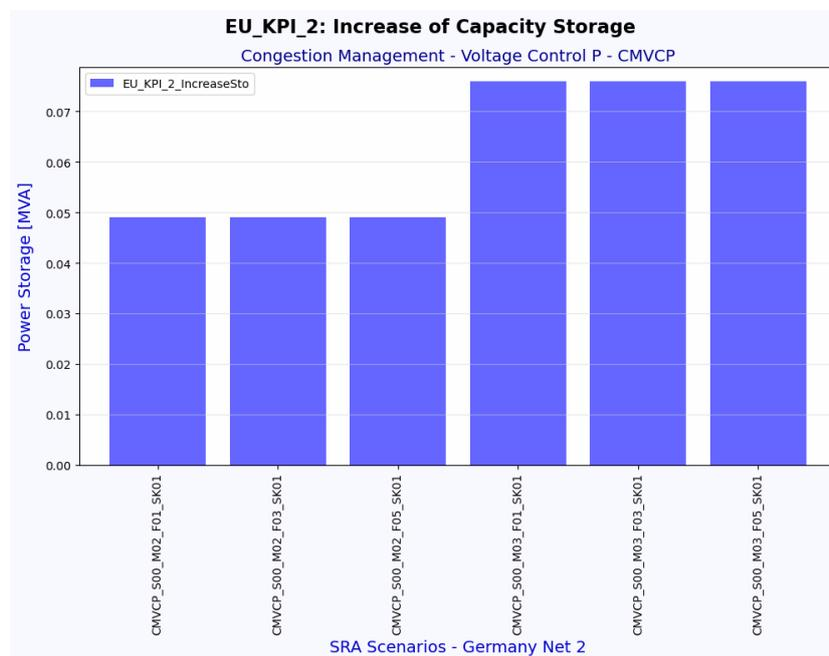
**Figure 2.105 EU\_KPI\_2: Increased of capacity storage solution, for Congestion Management, Voltage Control using Active Power (CMVCP)**
