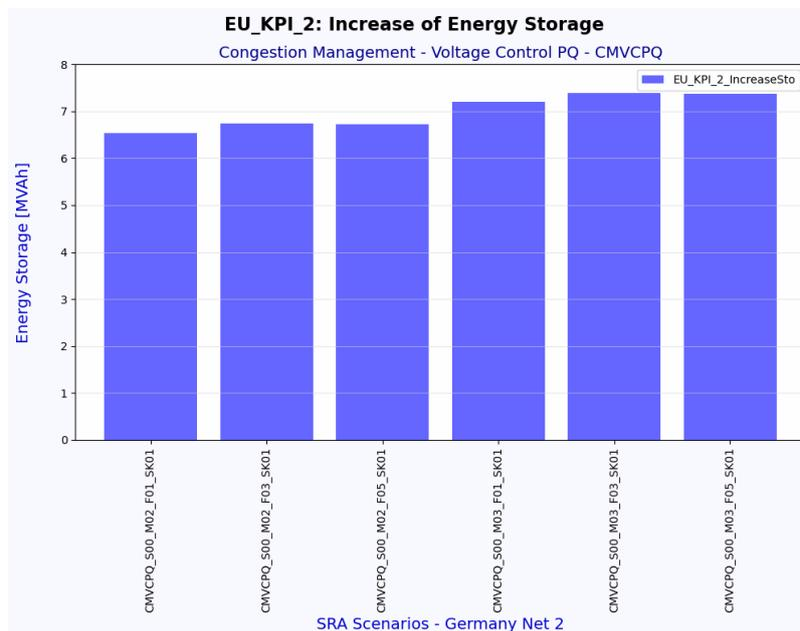
**Figure 2.111 EU\_KPI\_2: Increased of energy storage solution for Congestion Management, Voltage Control using Active and Reactive Power (CMVCPQ)**
