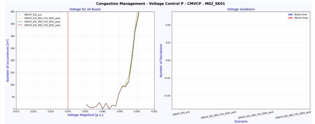
**Figure 2.30** Deviation plots for Voltage Magnitude [p.u.] obtained from Congestion Management – Voltage Control with Active Power (a) Scenario M01-K01, (b) Scenario M02-K01. Scenario 1, DE-NET1-LV.
